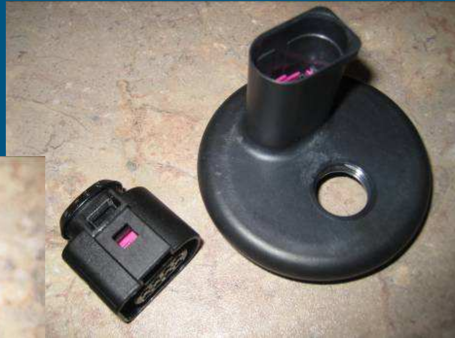
2X4 (8X MT2) Sealed Integrated Connector Cap for Emissions SCR Pump Motor End Cap with M16 thread boss for pressure fitting and retainer
